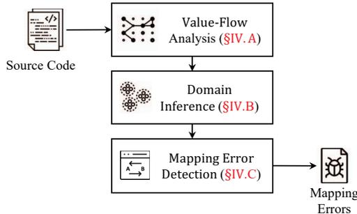
Fig. 3. System Overview of TRANSCODE
