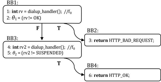
Fig. 5. The control-flow graph of function  $f_2$  in Figure 2
