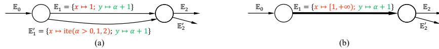
Fig. 6: Mixed abstract domain. (a) An example where we need to convert the precise symbolic domain to intervals. (b) After applying the mixed domain.
